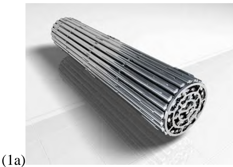
Figure 1: Picture of a CANDU ® nuclear fuel bundle with a schematic showing individual components. Bearing pads and spacers are coated with beryllium so that they can be brazed onto the zircaloy tubes.
